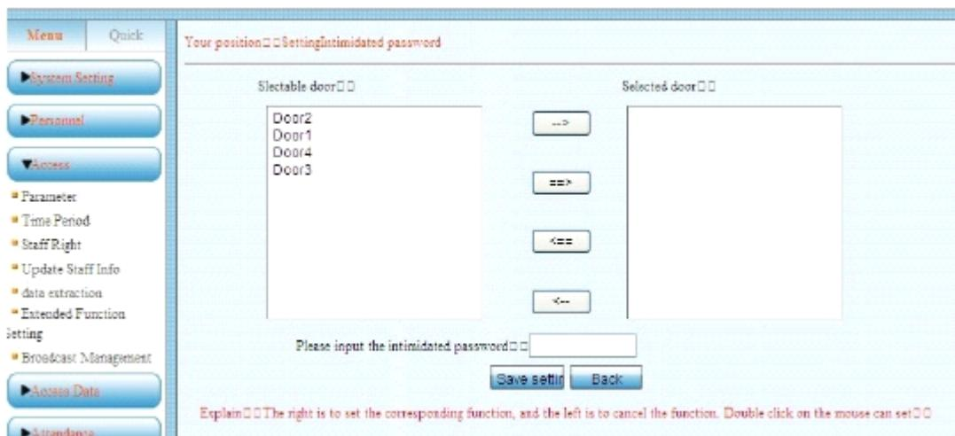
Can input one password as Intimidated password, this function is one person in the system intimidated by others, he can use this password open the door, the system will not alarm , but the system will have a intimidated alarm record.
